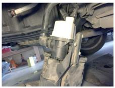
prevented me from removing it easily. I finally inserted the screwdriver between the pump and canister and pried upward
